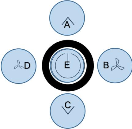
Menu navigation on the touch-surface is performed by pressing the buttons “up” (A), “down” (C), “left” (D), “right” (B) or the power button.
