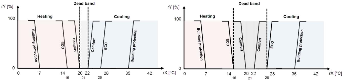
**Heating/ cooling with PI-controller (0..10 V) (only EC 3AO and EC AO2DO)**
